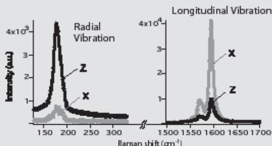
The radial breathing mode is detected effectively with z-polarization. ZPol provides a new detection technique sensitive to molecular orientation in 3D.
