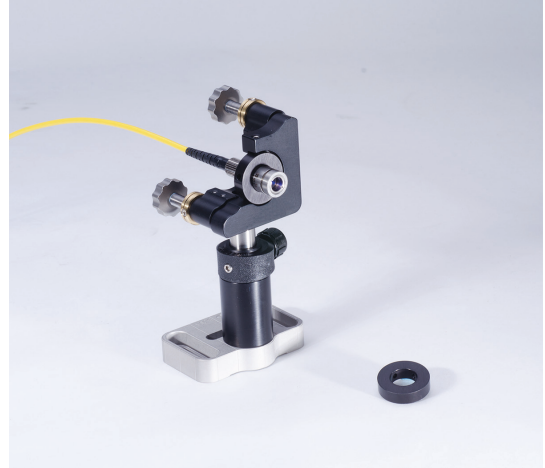
FC5 plus ring mounted in a 1 inch optical mount.
